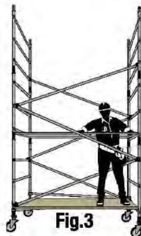
9. Install one platform as a temporary platform approximately 0.5m from the ground between both end frames. Install a ladder access platform approx 2m from the ground. See Fig. 3.
